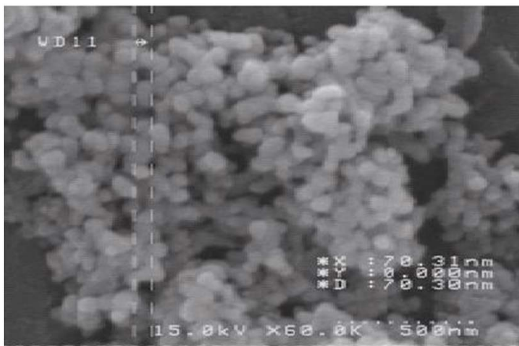
Fig. 4 SEM image of Ag/ Nylon 6,6 nanocomposites
